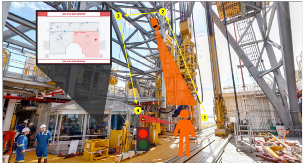
Cameras located above the drilling floor send real-time location information, enabling drivers to see when crew members have breached the red zone.
